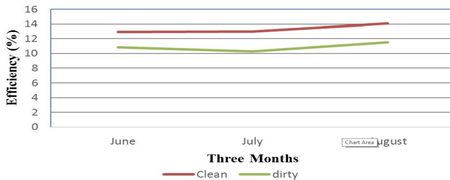
Figure 10. Efficiency comparison for clean and dirty polycrystalline PV modules
